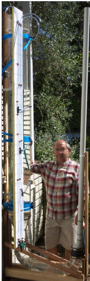
Fig 5: Apparatus before filling with sand; the Perspex column is full of water. The pipe on the right was to allow filling from the base under controlled conditions.
