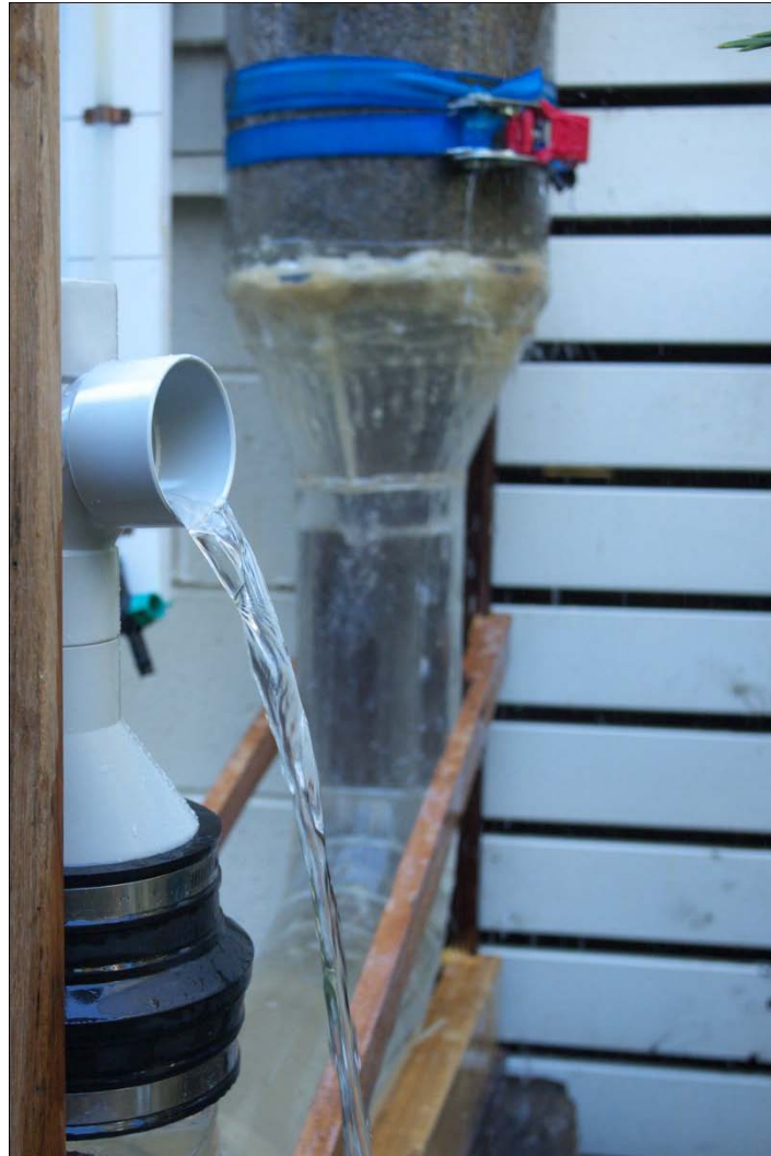
Fig 6: Final test; water allowed to cascade from base of column. The equilibrium position was that the water level at the outlet flow point (atmospheric pressure) was 35mm above the level into which the water from the column was cascading, presumably flow head converted to static head.
