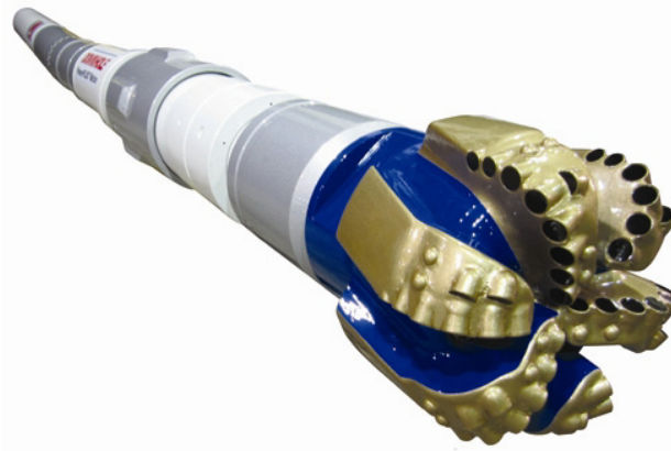
Figure 2a: Directional drill bit and motor
